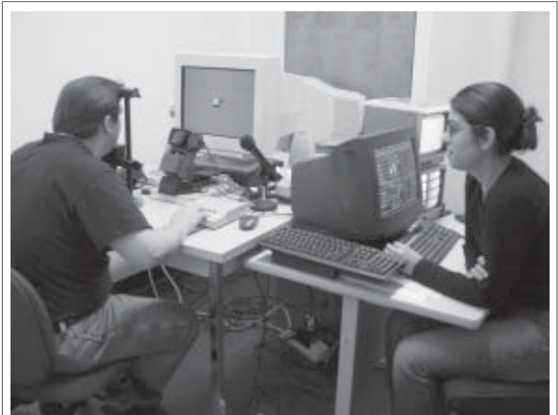
How do people direct their gaze when searching for objects? Psychology graduate students Dan Gajewski and Monica Castelhana demonstrate the eye-tracking machine that records eye movement patterns.
